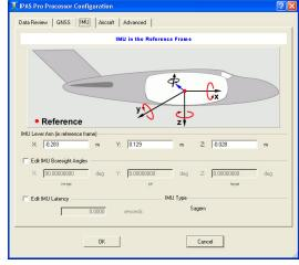
Leica IPAS Pro – Familiar and intuitive GNSS/IMU processing workflow
